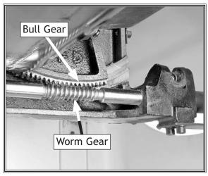
**Figure 84.** Location of the bull and worm gears.
